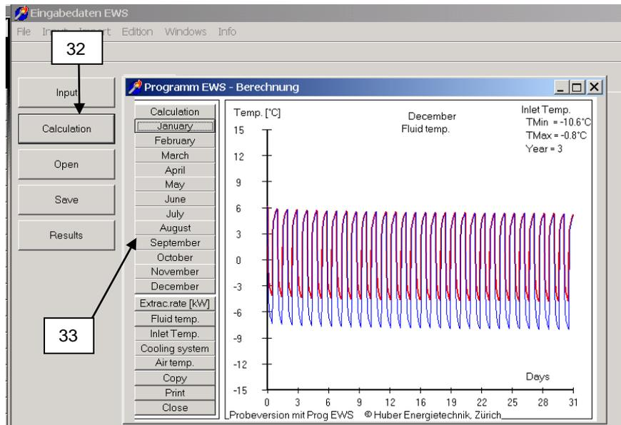
Fig. 5.1: Diagram of the inlet and outlet temperature of the fluid in December.
