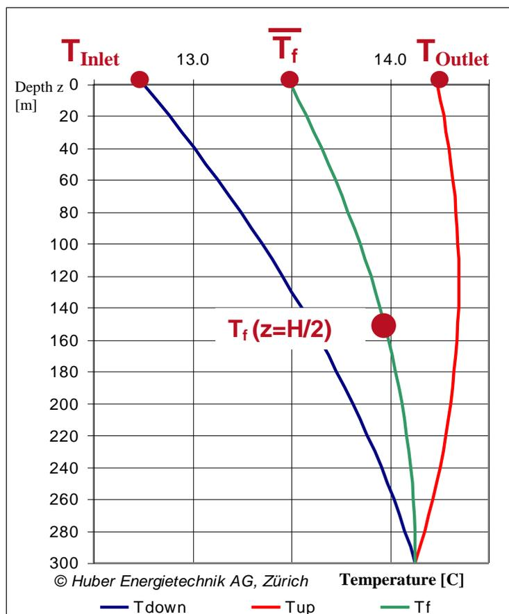
Fig. 6.8: Temperature profile of the fluid according to [9].
