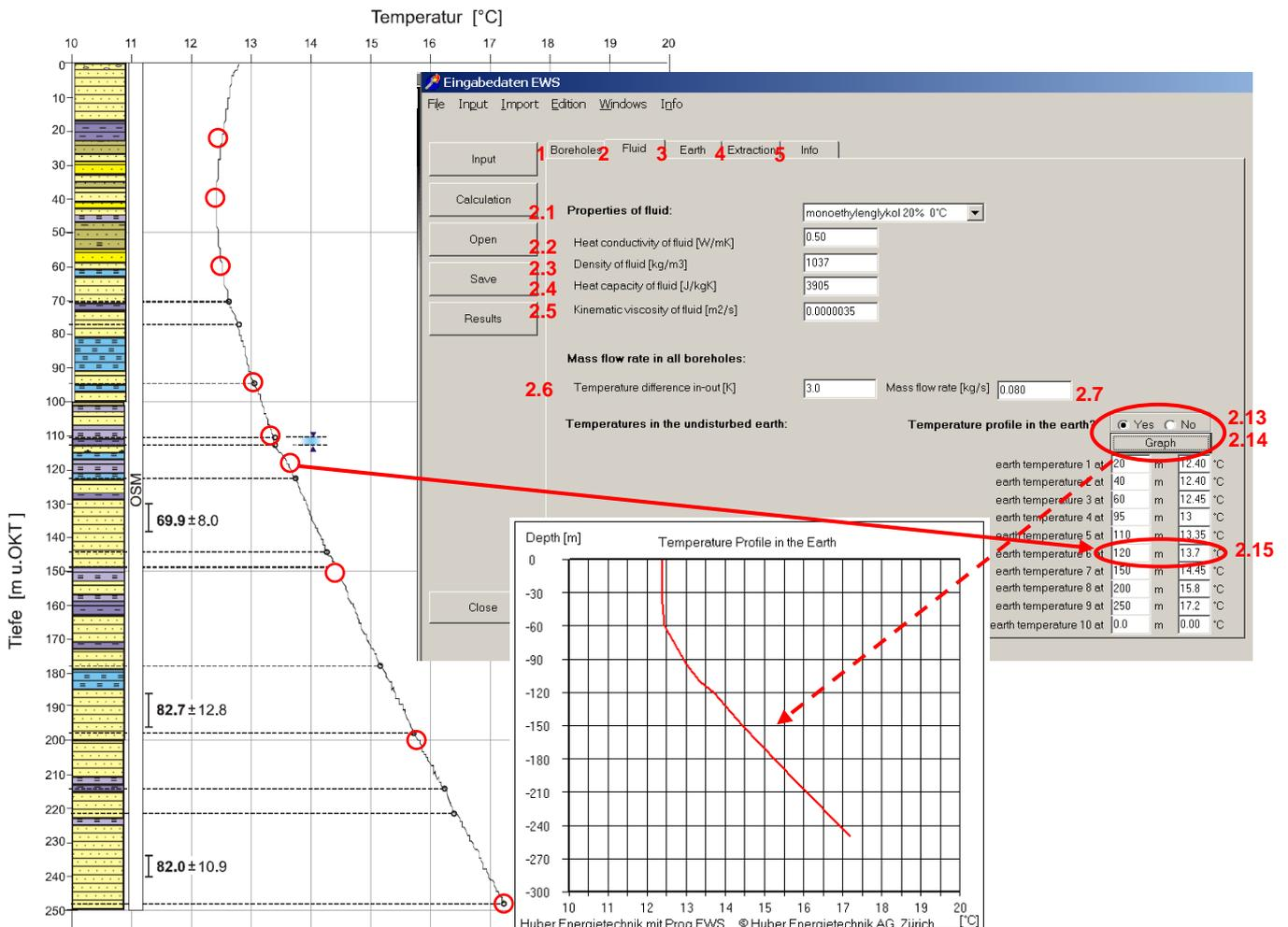
**Fig. 3.28: Input of the undisturbed temperature profile in the earth out of a measurement. (Example from a measurement of Dr. U. Schärli / E. Rohner [19]).**
