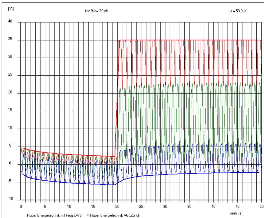
**Fig. 3.62: Change of load profile after 20 years of operation (addition of solar collectors to recuperate the boreholes). Minimum borehole inlet temperature rises to -2.3 °C after a total of 50 years.**
