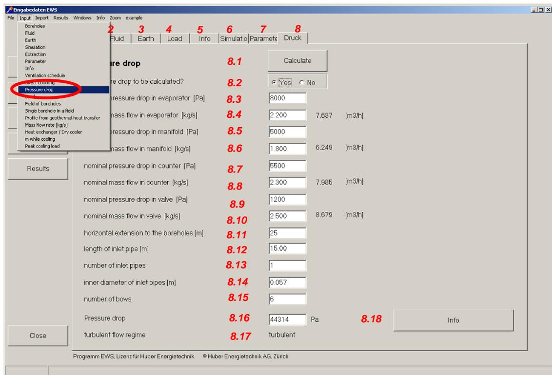
**Fig. 3.76:** The sheet “Pressure”.
