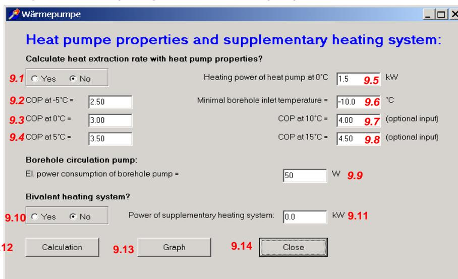
**Fig. 3.80:** The input mask of the heat pump properties and the additional heating system.
