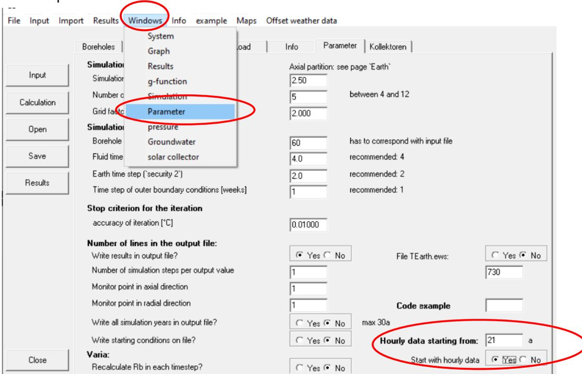
**Fig. 3.61: Sheet “Parameters”:** Starting the simulation with hourly data (prior to restauration measures) and a new load profile for the 21<sup>st</sup> year of operation and following.
