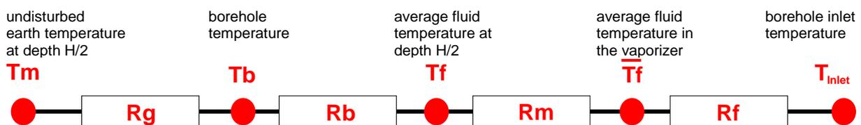
**Fig. 6.9** Thermal resistance of a borehole heat exchanger.
