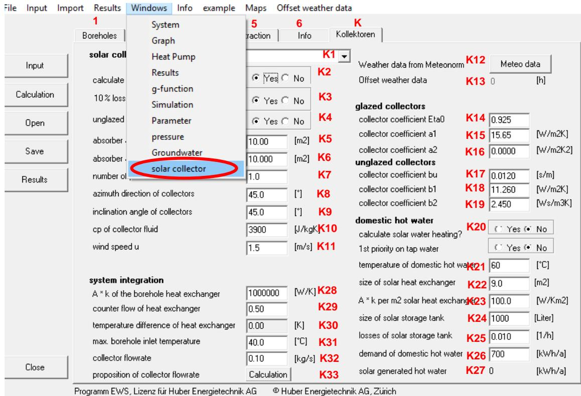
**Fig. 3.69:** Sheet "solar collectors" for the calculation of solar regeneration.
