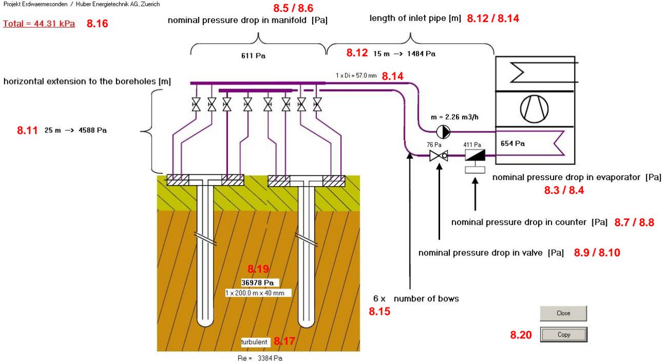
**Fig. 3.77: Display of the results in the borehole circuit**
