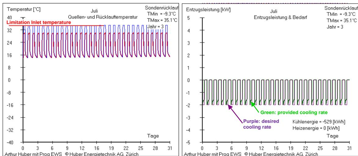
**Fig. 3.39: Limitation of the maximum borehole inlet temperature in the cooling case.**
