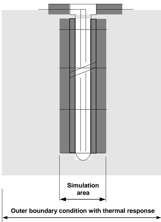
The Crank-Nicholson-method is used for the simulation of the ground temperatures close to the boreholes (1.5 - 3m).
