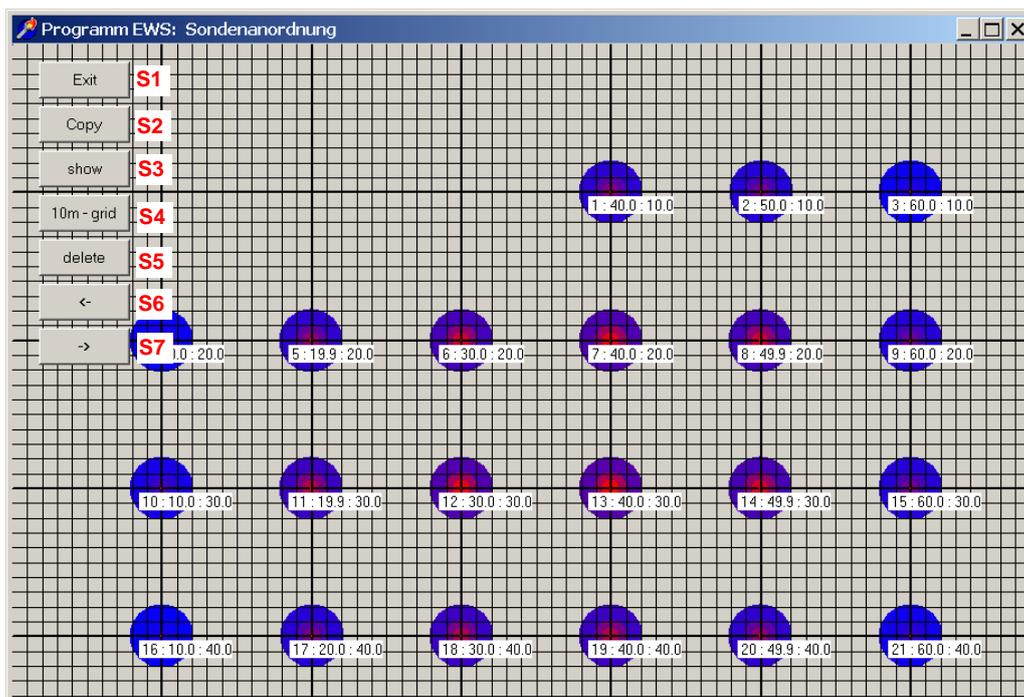
**Fig. 3.18:** The sheet “Field of boreholes” with 21 boreholes. The “blue” boreholes give a higher yield, the “red” boreholes give a lower yield.
