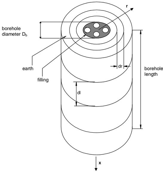
The calculations are done in an axially symmetric grid. The ground is divided in the axial direction into equal segments of the length  $dl$ .
