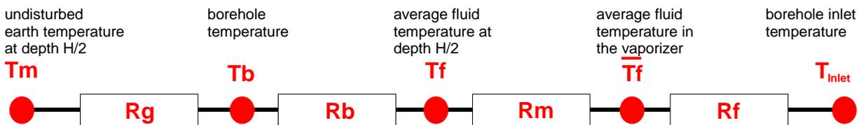
Fig. 6.7: Thermal resistance of a borehole heat exchanger systems
