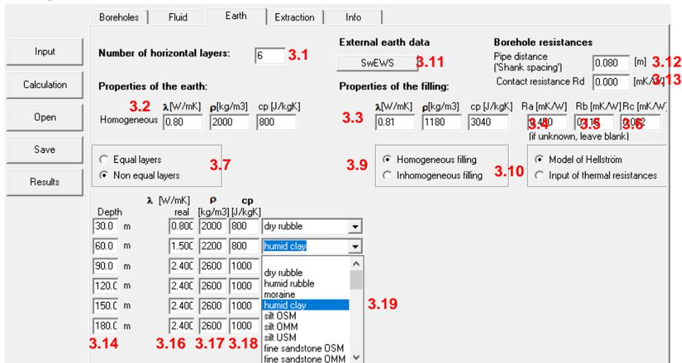
Fig. 3.33: The sheet „Earth“ offers a selection of rocks in the pull-down menu.
