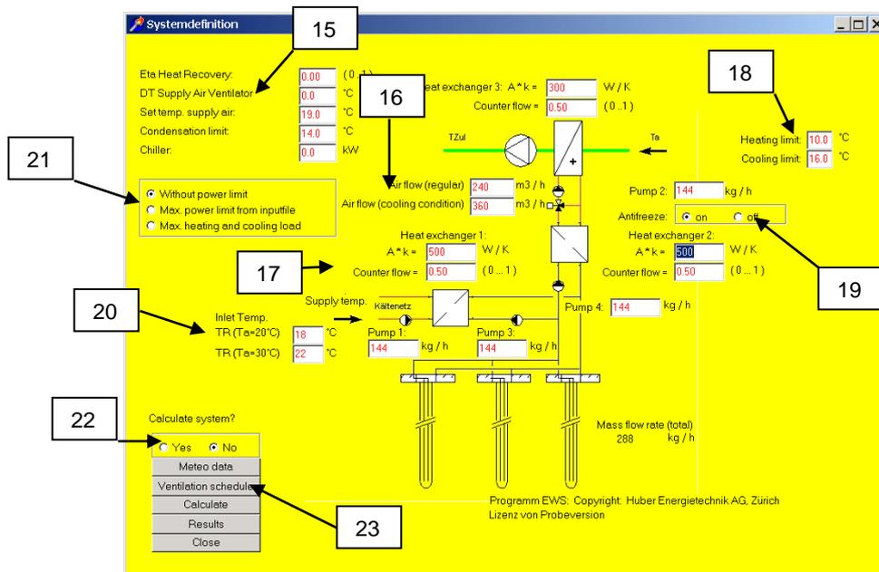
Fig. 3.82: The input mask “Systemdefinition” for direct cooling systems (without HP).
