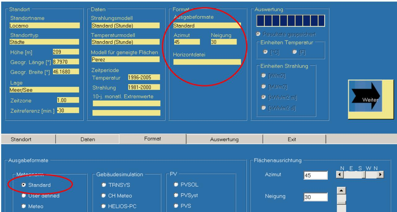
**Fig. 3.68:** Input of weather data, Azimuth (east= -90, south= 0°, west= 90°), slope and horizon in the program METEONORM [19]
