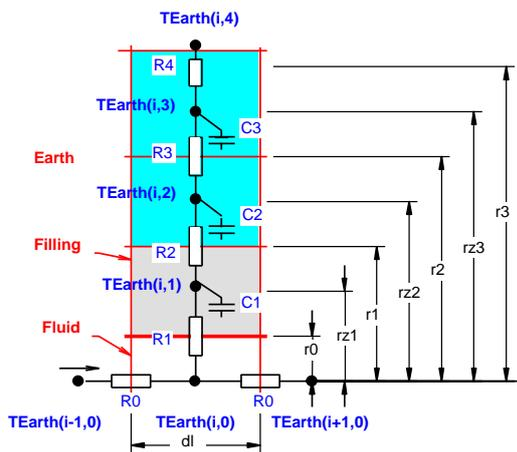
A grid factor of 2 doubles the difference of the radius between two calculation volumes.
