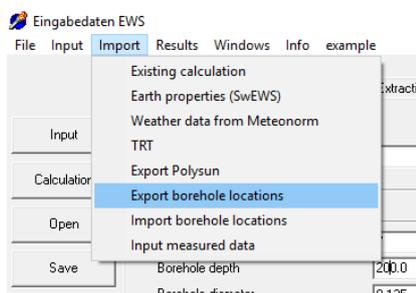
To save the borehole positions, one must exit the field of boreholes window and click the "Import" from the main menu, to then choose "Export borehole locations" and save this file to an appropriate folder.
