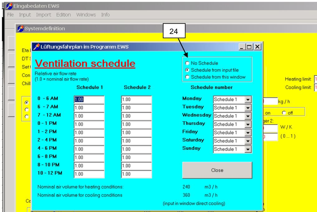
Fig. 3.83: The input mask “Ventilation schedule”.
