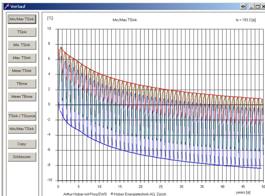
**Fig. 5.3: Graphical visualization of the sole temperature over the entire simulation period. In this example the monthly maximum (red), average (green) and minimum (blue) of the borehole inlet are represented.**
